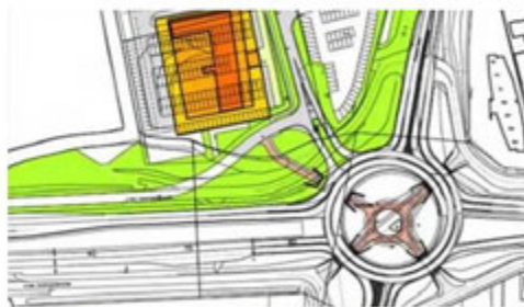
Figure 7 - Typical roundabout by-pass layout
