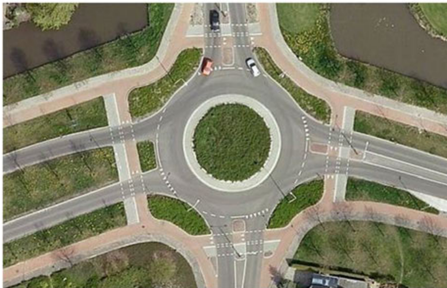
Figure 3 - Typical roundabout without cyclist priority
